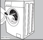
• Fill the smaller upper hole and the two large ones with the corresponding plastic plug caps supplied in the bag containing the instruction booklet.
